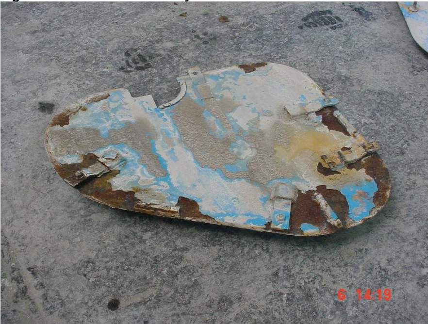
Figure 2: Side panel off loader after 6 year untreated
