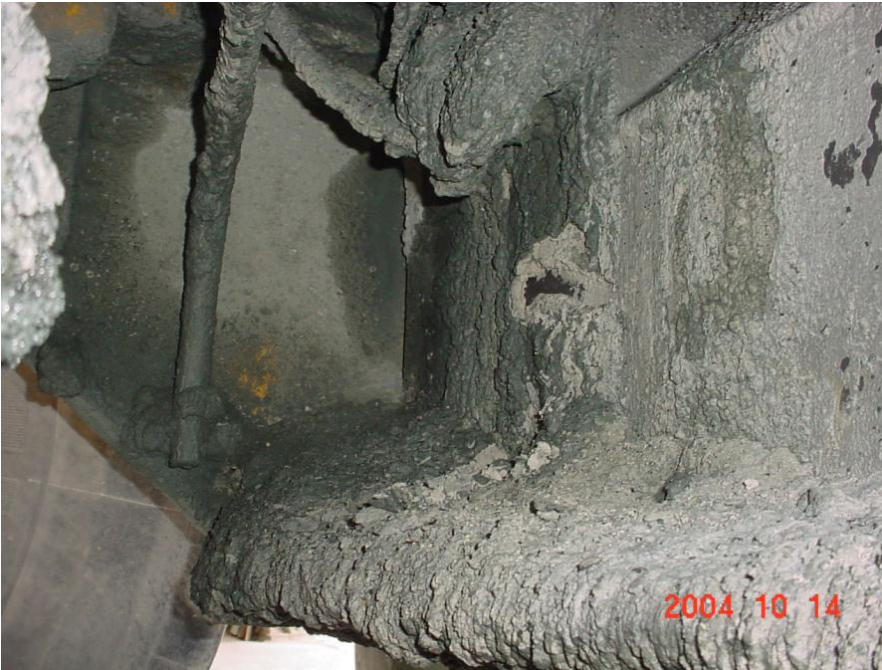
Figure 1: Under loader after 6 years not treated
