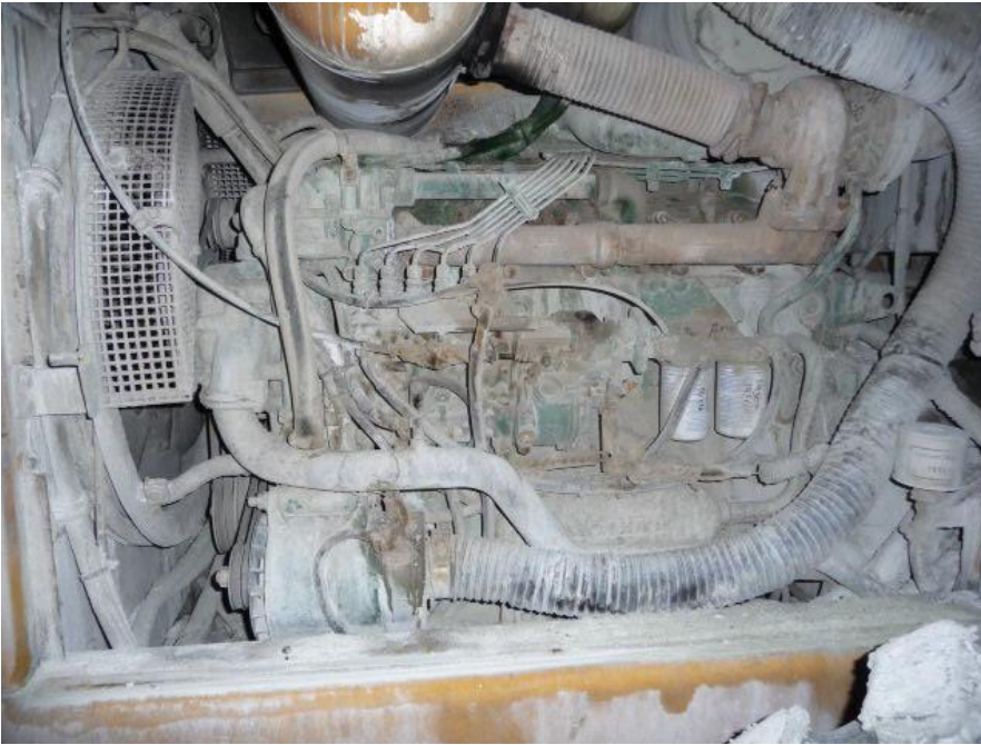
Figure 3: Engine bay after 6 years untreated (compare with Figure 11)
