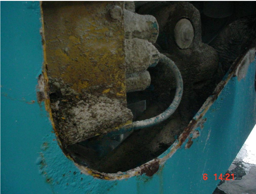
Figure 4: side of loader 6 years untreated (compare with Figure 10)
